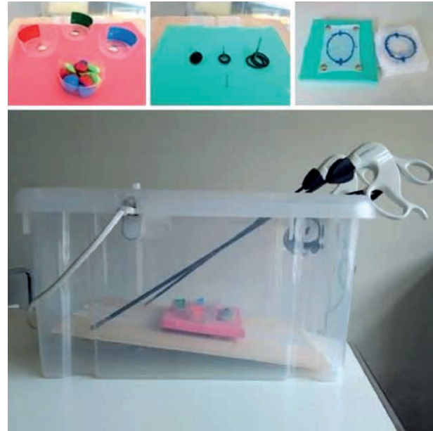
Figure 1. Custom-made simulator and exercise plates. A) Eye-hand coordination. B) Hand-hand coordination. C) Cutting. D) Final look of the custom-made simulator.
